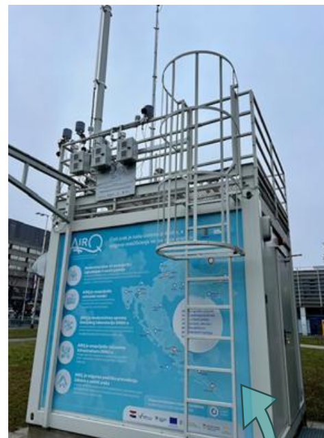
Zagreb-1 traffic measurement site with additional sensors installed
